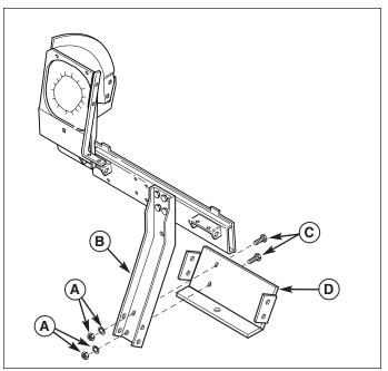
Figure 6. Assemble Catcher Frame (Prestige Shown)
